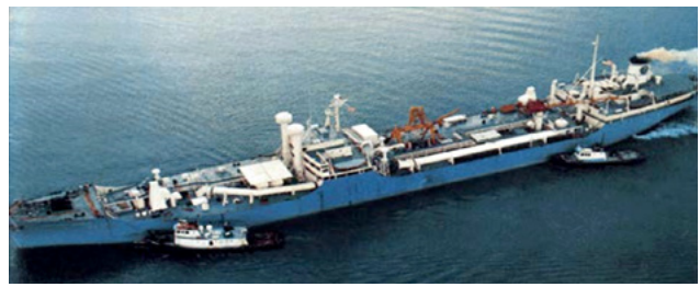
Figure 4.2 OTEC-1 facility in Honolulu (ex US Navy WW2 Turbo Electric T2 Tanker)
