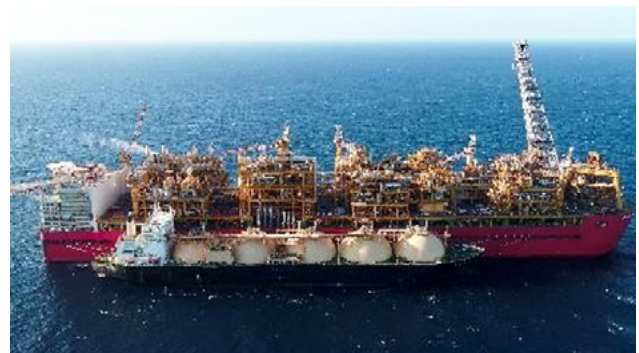
Figure 8.6 Shell's Prelude FLNG system with deep water intake risers shown at the Stern
